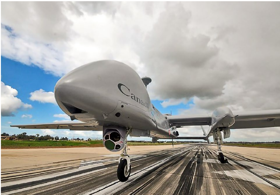
The L3Harris WESCAM MX™-20 EO/IR video camera will be part of the drone's sensor suite
